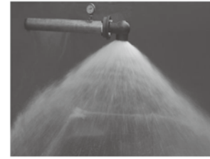
As a whole made of carborundum
